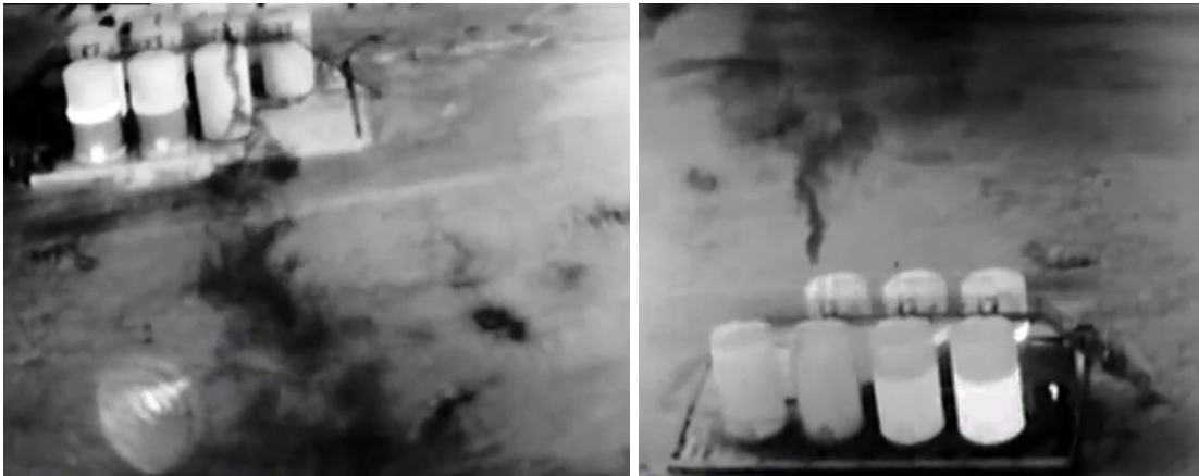
Infrared cameras can help detect gas leaks from production facilities such as this one located near Casper, Wyoming. (Photos: Environmental Defense Fund)
